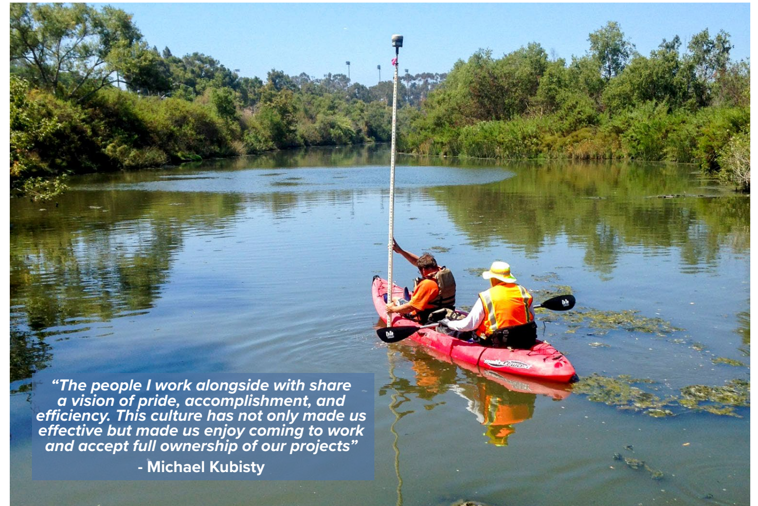
The Land Surveying Division record sediment build up and displacement to produce reporting for the San Diego Creek Scour Study Project prepared for Environmental Resources.
